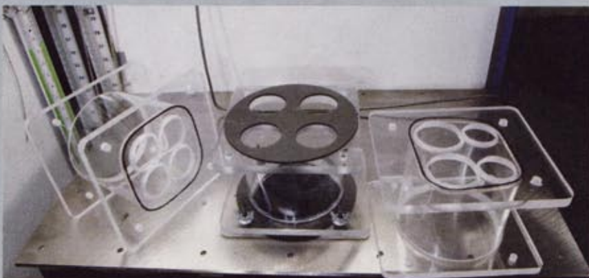
The adapter bases come in a variety of configurations to match the carb type, including 4150 squarebores, 4500 Dominators, and the spreadbore Quadrajet/ThermoQuad patterns. The entry side of the throttle bore simulators have a radiused form, providing airflow capacity exceeding the mightiest carb. O-rings provide the seal.
