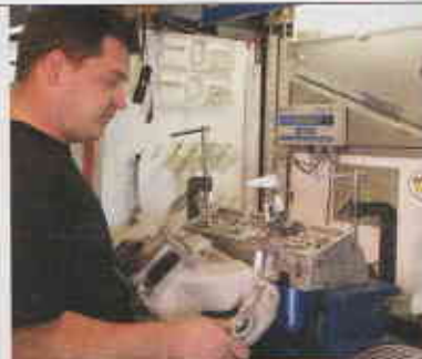
> To gain further insight into the airflow, all six of our manifolds were tested in conjunction with the cylinder head. In all cases, the porting improved the airflow of the head/manifold combination.
