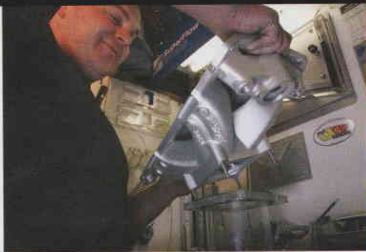
> Using a Dr. J's adapter and blowing into the plenum, Manifold Man Bryce Mulvey prepares to test an Edelbrock Super Victor intake. The flow adapter simulates the throttle bores of a 4150 carb.
